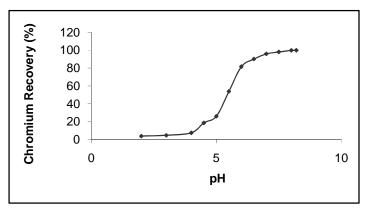
Fig. 1. Effect of pH on Chromium recovery from waste water.
