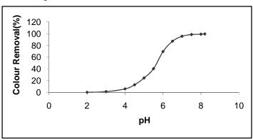
Fig. 2. Effect of pH on colour removal from waste water.
